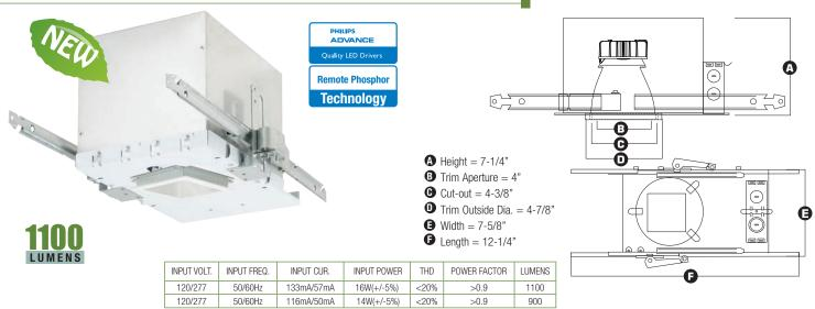
DESCRIPTION - 4" LED dedicated Architectural New Construction Downlight with integral LED heat management casting and driver (installed on junction box). Consuming less than 15 Watts and producing more than 900 usable lumens. Lighting is smooth and comfortable while using 30% less energy than the common 26W CFL downlight. Plus the eco-friendly Maxilume LED system features 70% lumen maintenance at 50,000 hours life, with Energy Star and California Title-24 (compliances pending).
