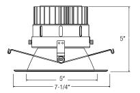
• Utilizes industry standard V or torsion springs, installs in most 6" and 5" incandescent down liahts.
