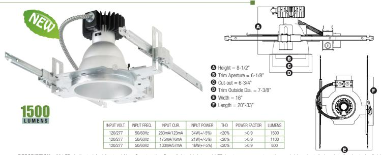
DESCRIPTION - 6" LED dedicated Architectural New Construction Downlight with integral LED heat management casting and driver (installed on junction box). Available in 800 lumens (16W), 1100 lumens (21W) & 1500 lumens (34W). Lighting is smooth and comfortable while using 25% less energy than the common 26W & 32W CFL downlight. Plus the eco-friendly Maxilume LED system features 70% lumen maintenance at 50,000 hours life, with Energy Star and California Title-24 (compliances pendina).
